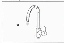
After installation is complete, remove aerator and rotate handle to the closed position. Turn on the water supply valves, and check all connections for a leak. Turn on your faucet and allow both hot and cold water to run at least one minute each. Replace Aerator.
