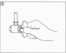
You should clean all the dirts from valve outlets. Turning off the water supply valves. This is usually found near the water meter. If you are replacing an existing faucet, remove the faucet from the sink and clean the sink surface thoroughly.
